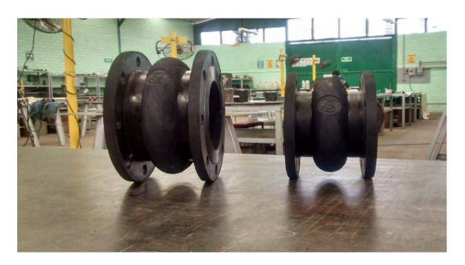
Expansion Joints are flexible devices designed to absorb movements generated by the pipe system because of variations in temperature and pressures. By absorbing those movements, the joints reduce the mechanical vibration caused by other equipment and diminishes the noise of the pipes.
