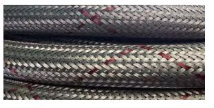
Coating made of plaited stainless steel wire that forms a protective mesh on the exterior of the hose, joint by a coated of welding with the hose and ring. This wire braid provides major resistance avoiding that it enlarges due to internal pressure. Double braid is possible to resist higher pressures.
